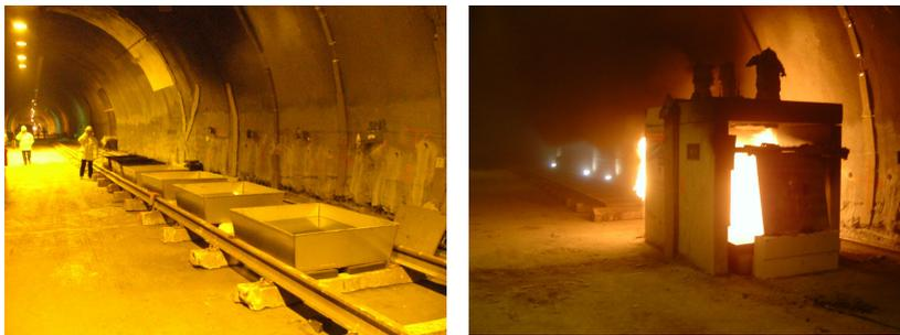
Fig.1. Fire pools on rail tracks used for heating the concrete surface of the Minitunnel (right picture)
