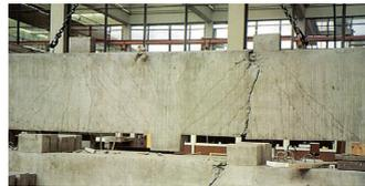
Fig. 3. Laboratory test of deep beam.
